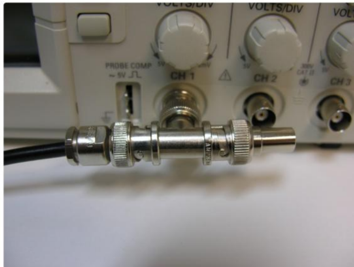
Figure 35: BNC T-Adapter on the oscilloscope with coaxial transmission line connected on the left and BNC 50 Ohm resistor connected on the right, to terminate the line.
